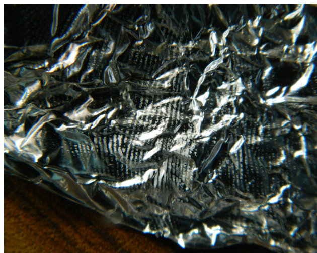
Figure 8 The developed latent fingerprint of grade 3 on crumpled aluminum foil (outer side) with the cyanoacrylate fuming.
