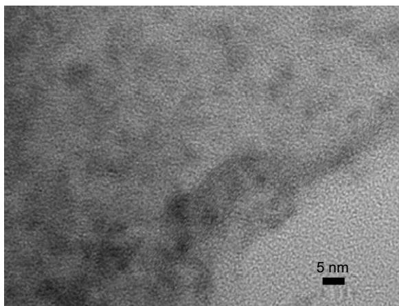
**Figure 2** Transmission electron microscopy image of GO-Fe<sub>3</sub>O<sub>4</sub> nanocomposites.
