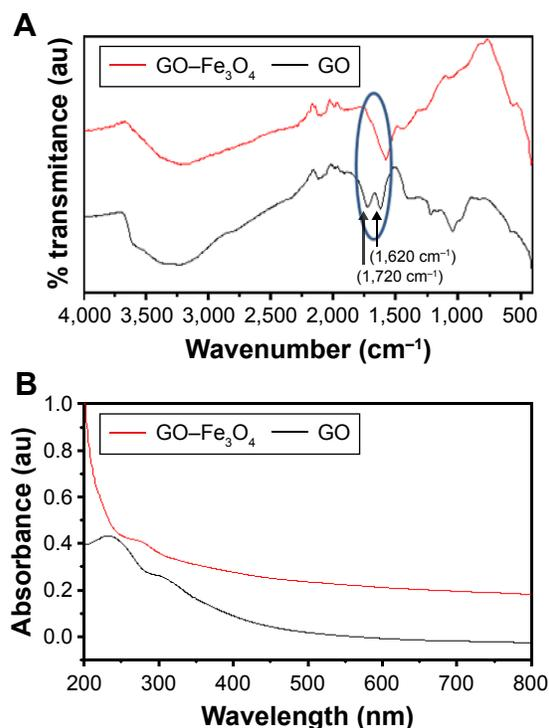
**Figure 1** (A) FTIR spectra of GO-Fe<sub>3</sub>O<sub>4</sub> nanocomposites and of pure GO. The circle area denotes the removal of IR bands in GO at (1720 cm<sup>-1</sup>), (1620 cm<sup>-1</sup>) on the formation of GO-Fe<sub>3</sub>O<sub>4</sub>. (B) UV–visible absorption studies of GO and GO-Fe<sub>3</sub>O<sub>4</sub> nanocomposites.
