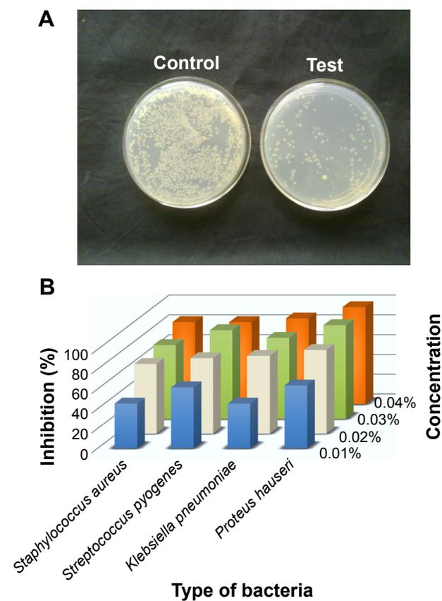
**Figure 3** (A) Colony-forming unit comparison of the sample GO-Fe<sub>3</sub>O<sub>4</sub> (0.02%) at 10<sup>-10</sup> dilution showing 76% inhibition of *Streptococcus pyogenes*. (B) Effects of the concentration of GO-Fe<sub>3</sub>O<sub>4</sub> nanocomposites on the bacterial growth.
